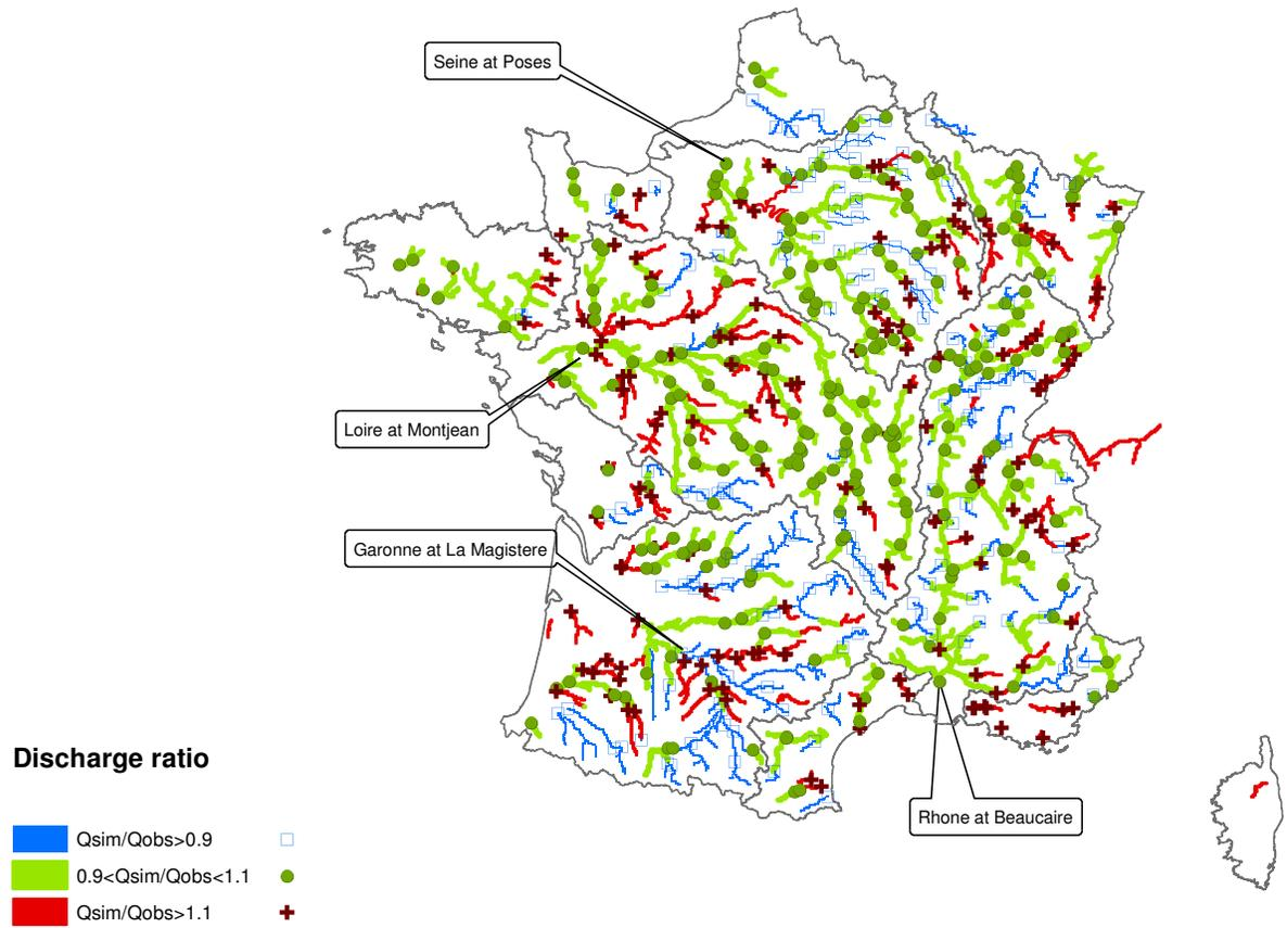
Figure 11. Spatial representation of the discharge ratio for each rivergages and the corresponding river network.
