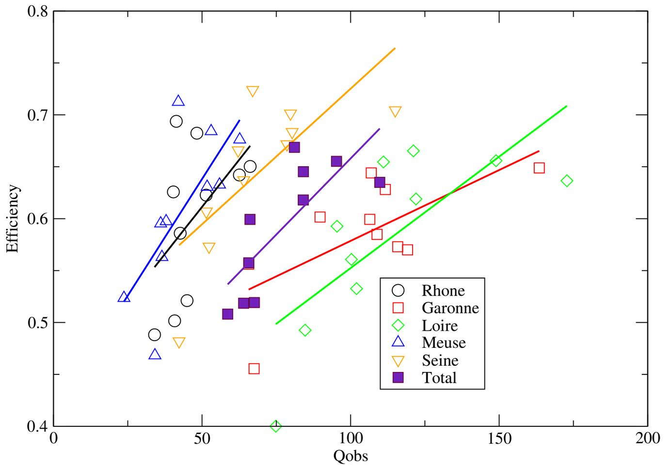
Figure 13. Relation between the efficiency and the observed discharge on average on the selected rivergages of each basin. The line correspond to the linear regression for a given basin
