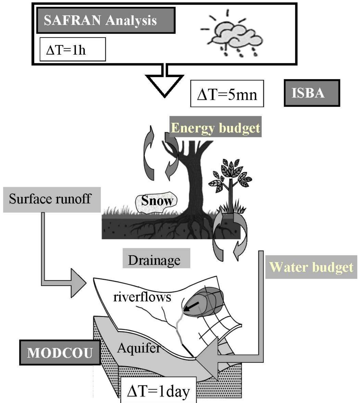
Figure 1. The SIM hydrometeorological model consists in three independent modules: the SAFRAN atmospheric analysis, the ISBA land surface model, and the MODCOU hydrogeological model
