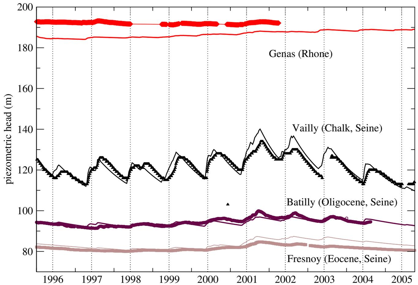
Figure 15. Evolution of the observed (symbol) and simulated (line) piezometric head for one given station over each layer of the Seine and Rhone aquifers
