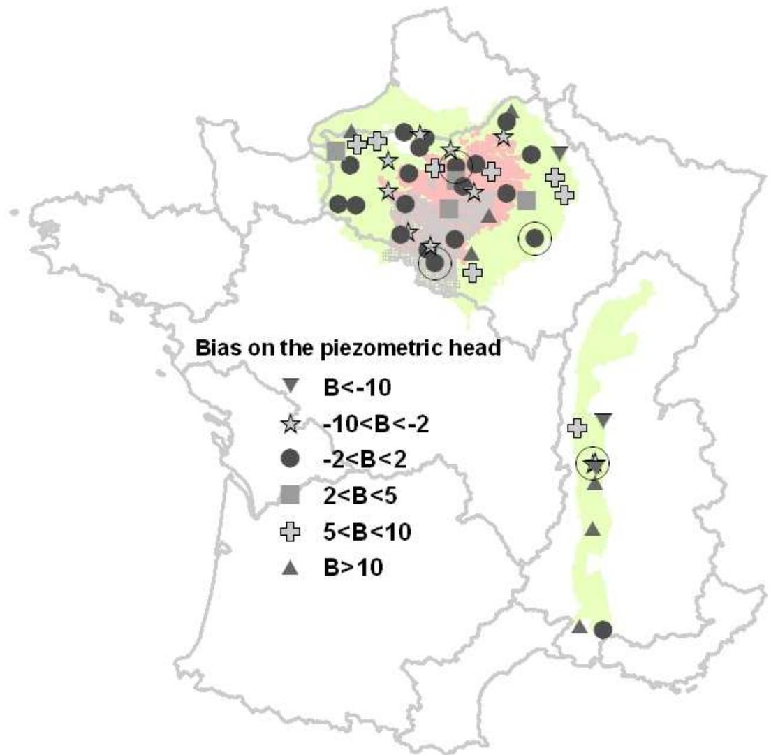
Figure 14. Spatial distribution of the bias on the 10-year simulation of the piezometric head simulated by SIM
