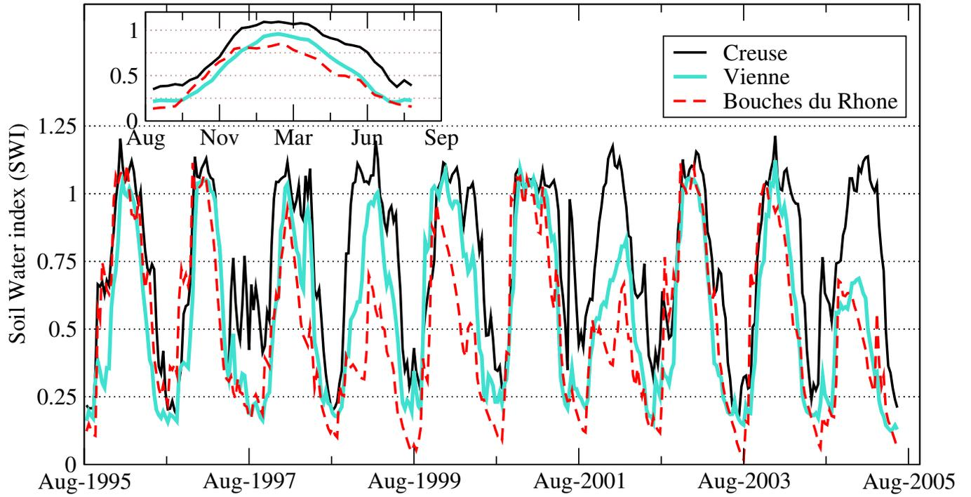
Figure 20. 10-day evolution of the soil water index (SWI) on the 3 sites plotted in figure 19. The encapsulated graph is the annual average
