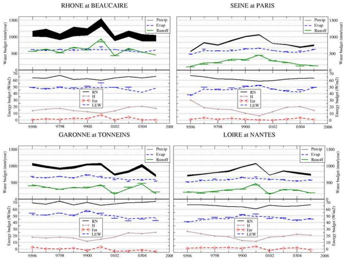
Figure 18. Water and energy budgets over the 4 main basins. The thick black lane is the total precipitation (Precip), and its thickness represents the snowfall. Evaporation (Evap), total runoff (Runoff) and latent heat flux (LEW) have an error bar that was estimated according to the error between the observed and simulated discharge. This error is shown in the energy budget panel (bottom panel) (Err) in order to compare with the net radiation (RN) and the sensible heat flux (H).
