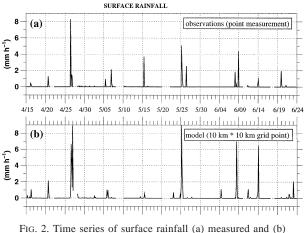
FIG. 2. Time series of surface rainfall (a) measured and (b) simulated at the Central Facility (3-h-mean values).
