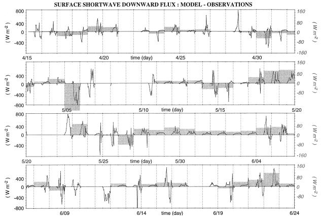
FIG. 10. Time series of differences between simulated and measured surface shortwave downward flux (30-min average values) for period 15 Apr-24 Jun 1998. Gray shading indicates 24-h average values, using the *y* axis on the right-hand side.
