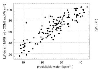
FIG. 14. Scatterplot of the differences between clear sky longwave flux at the surface simulated by the MM5 and CCM3 radiative schemes as a function of precipitable water (offline test for 14 clear sky days, 112 points).
