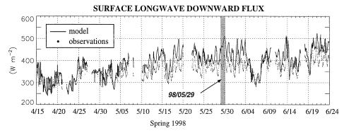
FIG. 13. Time series of simulated (solid line) and observed (dots) surface longwave downward flux (30-min-mean values). Gray shading indicates the day chosen for in-line sensitivity tests of the radiation scheme.
