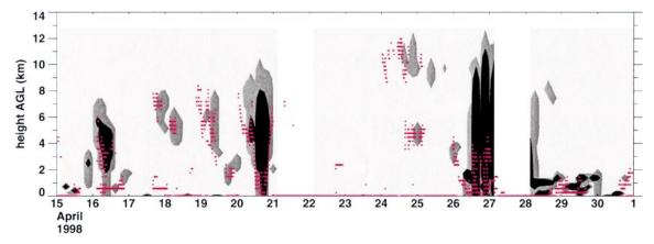
FIG. 7. Time–height cross section of simulated hydrometeor mixing ratio for the period 15–30 Apr 1998 (3-h sampling) and cloud-base heights (small red dots) measured by the micropulse lidar at the Central Facility (1-min sampling, data missing for part, of 15, 17, 29, and 30 Apr); light gray, gray, and black shadings correspond to hydrometeor mixing ratio values lower than  $10^{-6}$ , between  $10^{-6}$  and  $10^{-4}$ , and higher than  $10^{-4}$  kg kg<sup>-1</sup>, respectively.
