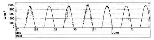
FIG. 12. Time series of observed surface shortwave downward flux at the Central Facility from 27 May to 3 Jun 1998 (1-min sampling).
