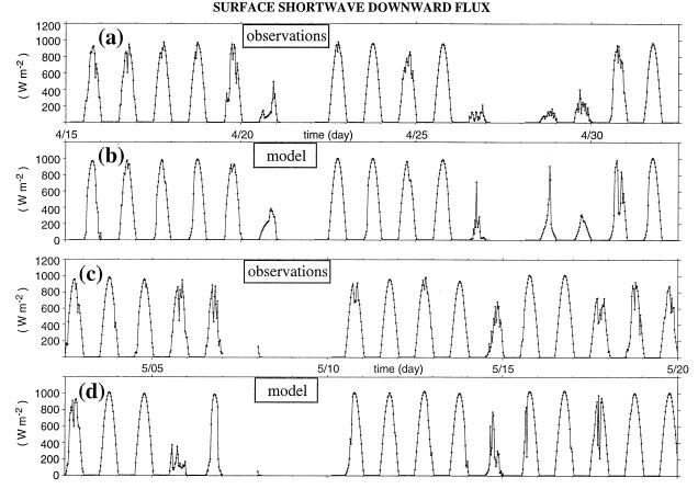
FIG. 9. Time series of (a), (c), (e), and (g) observed and (b), (d), (f), and (h) simulated surface shortwave downward flux (30-min average values) for period 15 Apr-24 Jun 1998.
