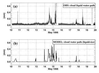
FIG. 8. Time series of 1-min-mean of (a) cloud liquid water path measured by the microwave water radiometer at the Central Facility and of (b) cloud liquid water path, including ice cloud water, simulated by MM5 for the period 10–20 May 1998.
