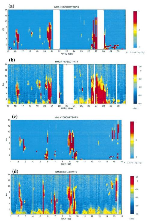
FIG. 6. Time-height cross section of (a) simulated hydrometeor mixing ratio and (b) radar reflectivity measured by the millimeter wave cloud radar (best reflectivity estimate) for the period 15–30 Apr; (c), (d), (e), (f), and (g), (h) same as (a), (b) except for the periods 1–15 May, 16–31 May, and 1–16 Jun 1998, respectively (3-h sampled instantaneous values).
