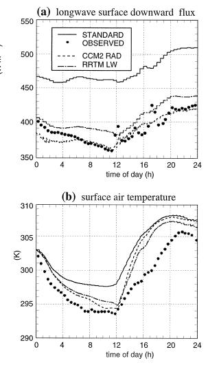
FIG. 15. Comparison with observations of (a) the longwave downward flux and (b) the air temperature at the surface simulated by MM5 for the 29 May 1998 with three different radiative schemes.
