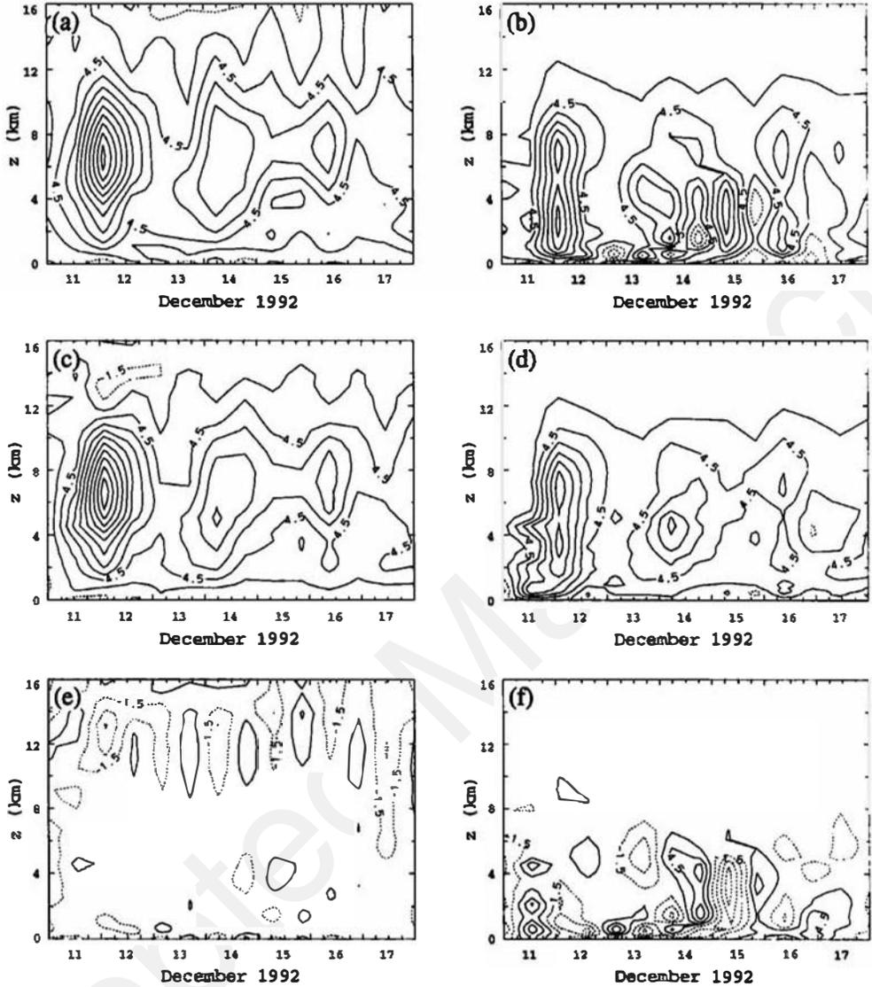
Figure 4. Temporal evolution of (a) the apparent heat source  $Q_1$  and (b) apparent moisture sink  $Q_2$  diagnosed from observations, (c) and (d) simulated  $Q_1$  and  $Q_2$ , and (e) and (f) differences between simulated and observed. The contour interval is  $3 \text{ K d}^{-1}$  starting from the 1.5 isoline (not the zero isoline) and the time average is 6 h.
