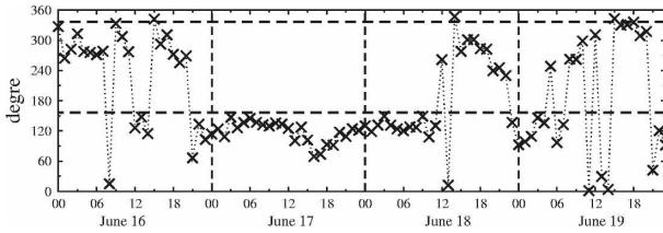
FIG. 5. The wind direction ( $^{\circ}$ ) at the tower top at Basel-Sperrstrasse from 16 to 19 Jun. The dashed horizontal lines indicate the directions ( $160^{\circ}$  and  $340^{\circ}$ ) perpendicular to the street canyon.
