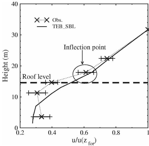
FIG. 3. The average vertical profile of wind speed, normalized by  $u(z_{\text{for}})$  at the tower top during the first half of the IOP in the frame of BUBBLE, for measurements and TEBSBL. Data source: Sonic, 600-s time step, neutral stability at tower top, and calm situations with a mean wind speed lower than  $1 \text{ m s}^{-1}$  at top level are excluded. The bars present the std dev of the observations.
