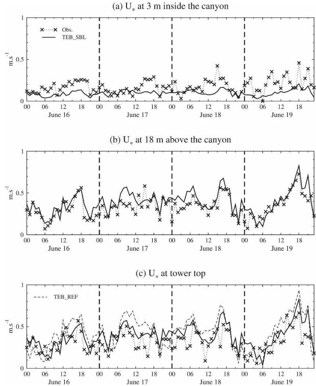
FIG. 9. Time variation of the friction  $U_*$  from 16 to 19 Jun in the street canyon at (a) 3 m AGL, (b) 18 m AGL (i.e., above the canyon), and (c) the tower top for TEB\_SBL and measurements. In (c) we present also the friction velocity calculated with TEB\_REF at tower top.
