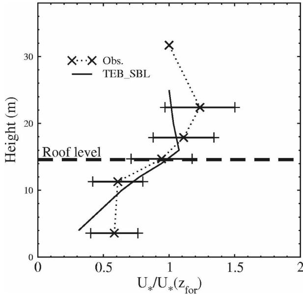
FIG. 8. The average profile of the local friction velocity normalized by its value at tower top  $U_*(z_{for})$  for TEB\_SBL and measurements. The profiles are averaged using 600-s time step data obtained during the first half of the IOP (15 days) for all stabilities. The bars present the std dev of the observations.
