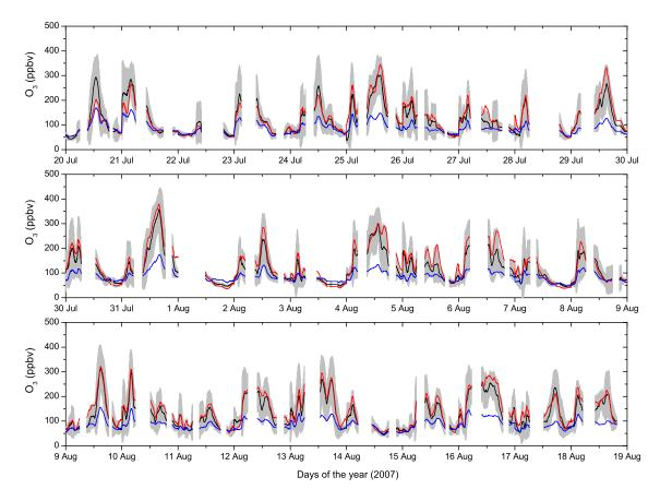
**Fig. 5.** Time-series of collocated MLS  $O_3$  assimilated field (black) with its standard deviation (shaded colour) compared to MOZAIC measurements (red) and model free run output (blue) for the period: 20 July–19 August 2007. Only observations above the altitude pressure of 280 hPa are used for the comparison, since we are interested in the tropopause layer (the cruise flight altitude pressure of MOZAIC aircraft is around 200 hPa). Units: parts per billion by volume (ppbv).
