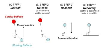
Fig. 1. Principle of the dual-balloon sounding.
