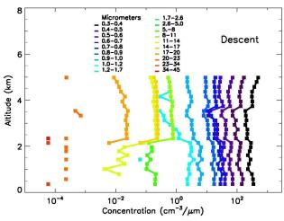
**Fig. 11.** Vertical profiles of aerosol concentration as a function of particle size inferred from the LOAC probe between 09:00 and 09:45 UTC on 23 September 2012. Upper (lower) panel shows data collected during the ascending (descending) phase of the sounding.
