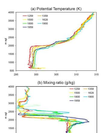
**Fig. 6.** Time series of hourly soundings performed on 1 July 2011 between 13:00 and 20:00 UTC. (a) Potential temperature (K) and (b) water vapour mixing ratio (g kg<sup>-1</sup>). Bold and thin lines correspond to ascending and descending soundings, respectively.
