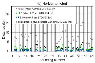
**Fig. 7.** Difference between actual and simulated radiosonde falling points as a function of (a) ascent rates and (b) horizontal wind profiles used to simulate the trajectories. Scores are computed for recovered balloons only.
