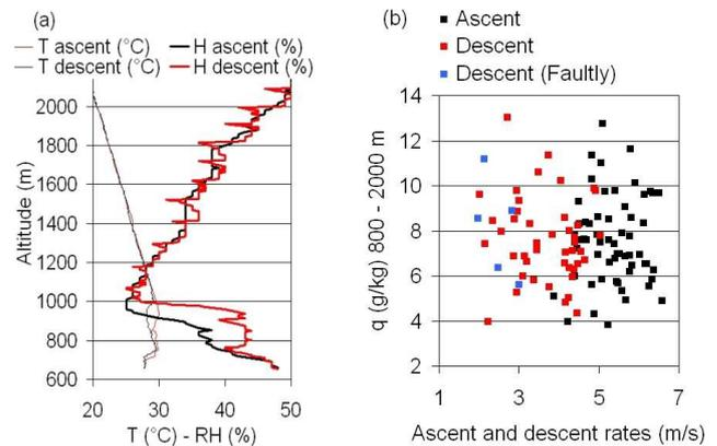
**Fig. 8.** Effect of insufficient ventilation on radiosonde measurements. (a) Example of disturbed sounding made during BLLAST on 26 June 2012, at 20:08 UTC. (b) Ascent and descent rates vs. mean specific humidity (g kg<sup>-1</sup>) between 800 and 2000 m for ascending soundings (black), descending soundings (red) and disturbed descending soundings (blue).
