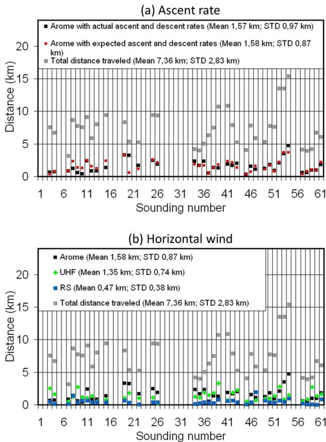
**Fig. 7.** Difference between actual and simulated radiosonde falling points as a function of (a) ascent rates and (b) horizontal wind profiles used to simulate the trajectories. Scores are computed for recovered balloons only.
