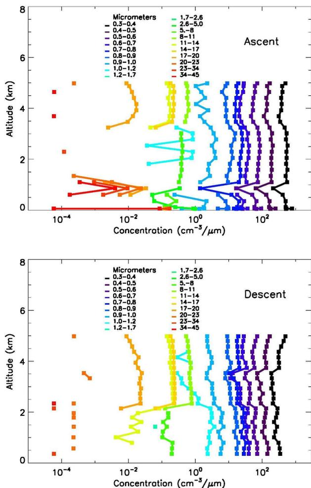
**Fig. 11.** Vertical profiles of aerosol concentration as a function of particle size inferred from the LOAC probe between 09:00 and 09:45 UTC on 23 September 2012. Upper (lower) panel shows data collected during the ascending (descending) phase of the sounding.
