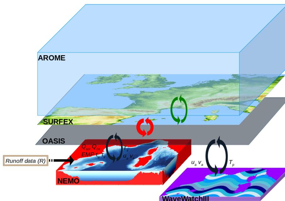
**Figure 1.** The NEMO-AROME-WW3 coupled architecture and domains illustrated by orography (of the AROME-France domain in the SURFEX “area”) and the NWMED72 bathymetry (in the NEMO box). The SURFEX-OASIS interface (red arrows) is detailed in Voldoire et al. (2017), and the AROME-SURFEX links (green arrows) are described in Masson et al. (2013) and Seity et al. (2011). See text and Table 1 for the exchanges involving NEMO and WW3.
