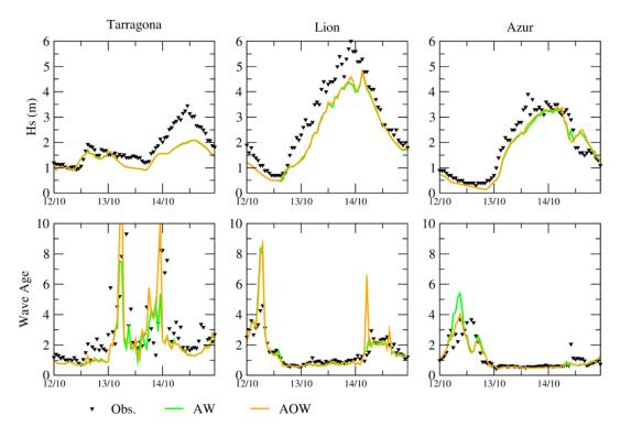
Figure 9. Time series of simulated significant wave height  $H_s$  and wave age at the three moored buoys Tarragona, Lion and Azur at 00:00 UTC on 12 October to 00:00 UTC on 15 October, using successive forecasts of each experiment including WW3 (+1-+24 h forecast ranges each day).
