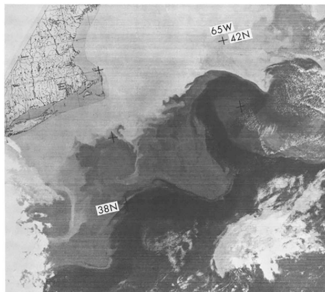
Fig. 8. VHRR IR image 4531 from NOAA 4 was obtained on November 12, 1975. The Gulf Stream north of Cape Hatteras and south of Cape Cod appears as the warmest (darkest) water. The large amplitude meanders as well as two warm core eddies are evident south of Cape Cod and Long Island (Legeckis, 1978).
