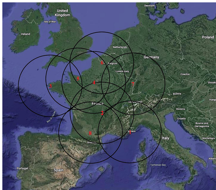
Fig. 4. Météo-France ADS-B antenna network (reception range \sim 400 km). See Table 3 for exact positioning.
