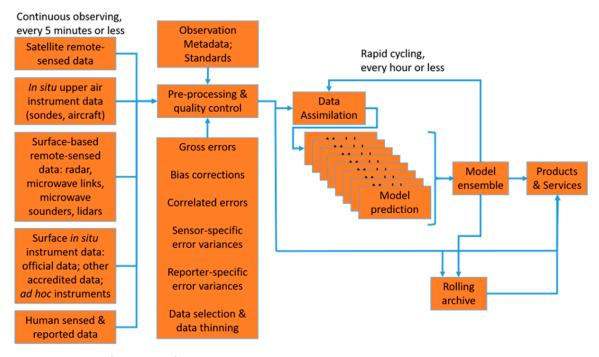
Fig. 7. Outline of the data flow in a kilometer-scale rapid update prediction system. Very short-range forecasts will be based on the latest observations or on the most recent NWP cycle. Longer forecasts may use multiple NWP cycles to optimize ensemble spread.
