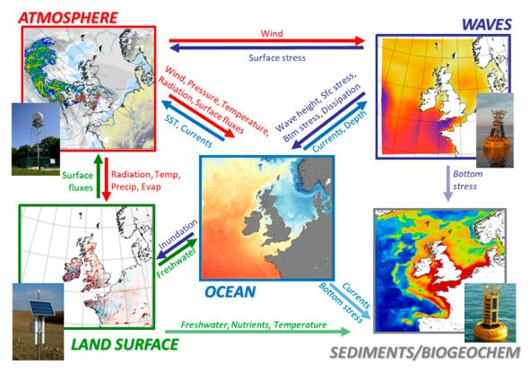
Fig. 8. Concept diagram of the U.K. Environmental Prediction (UKEP) coupled modeling project (H. W. Lewis 2018, personal communication). Progress to date is described in Lewis et al. (2018).
