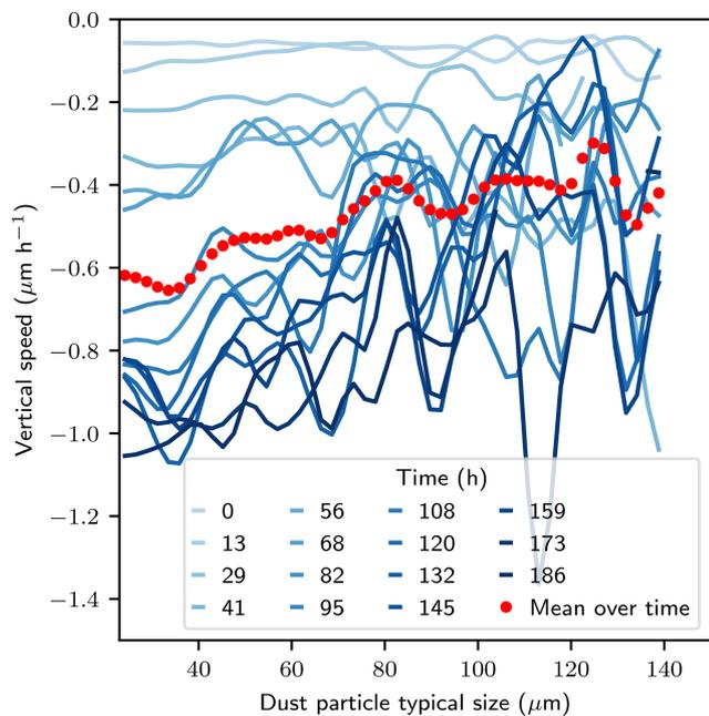
**Figure A3.** Mean vertical speed as a function of dust particle size for the temperature gradient experiment. Note that, here, only movements of type 1 and 2 and particles of volumes larger than  $5^3$  voxels were taken into account.
