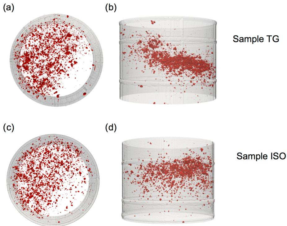
**Figure A1.** A 3-D view of the initial dust location (red) in the temperature gradient experiment (**a**, **b**) and the isothermal experiment (**c**, **d**) from top view (**a**, **c**) or side view (**b**, **d**). The aluminum sample holder inner contour is shown in transparent gray. The scale is indicated by the sample holder inner diameter, which is 10 mm.
