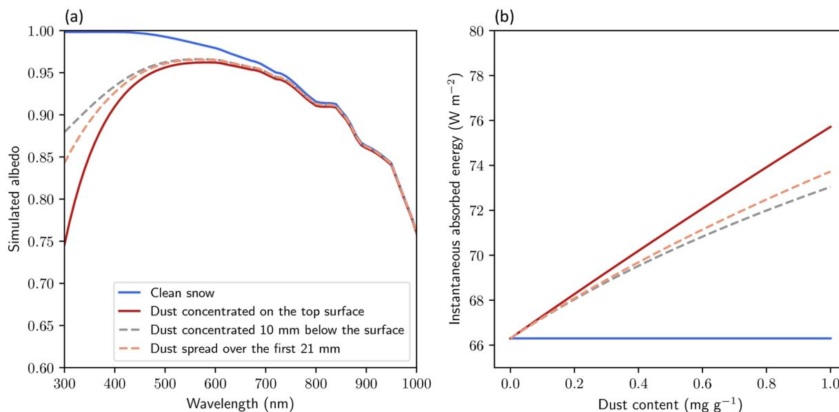
**Figure 6.** Simulated impact of dust motion on snow radiative properties. **(a)** Albedo as a function of wavelength for different idealized snowpacks and an initial dust concentration of  $1 \text{ mg g}^{-1}$ . **(b)** Instantaneous absorbed energy at a  $70^\circ$  solar zenith angle as a function of the initial dust content and for the same idealized snowpacks.
