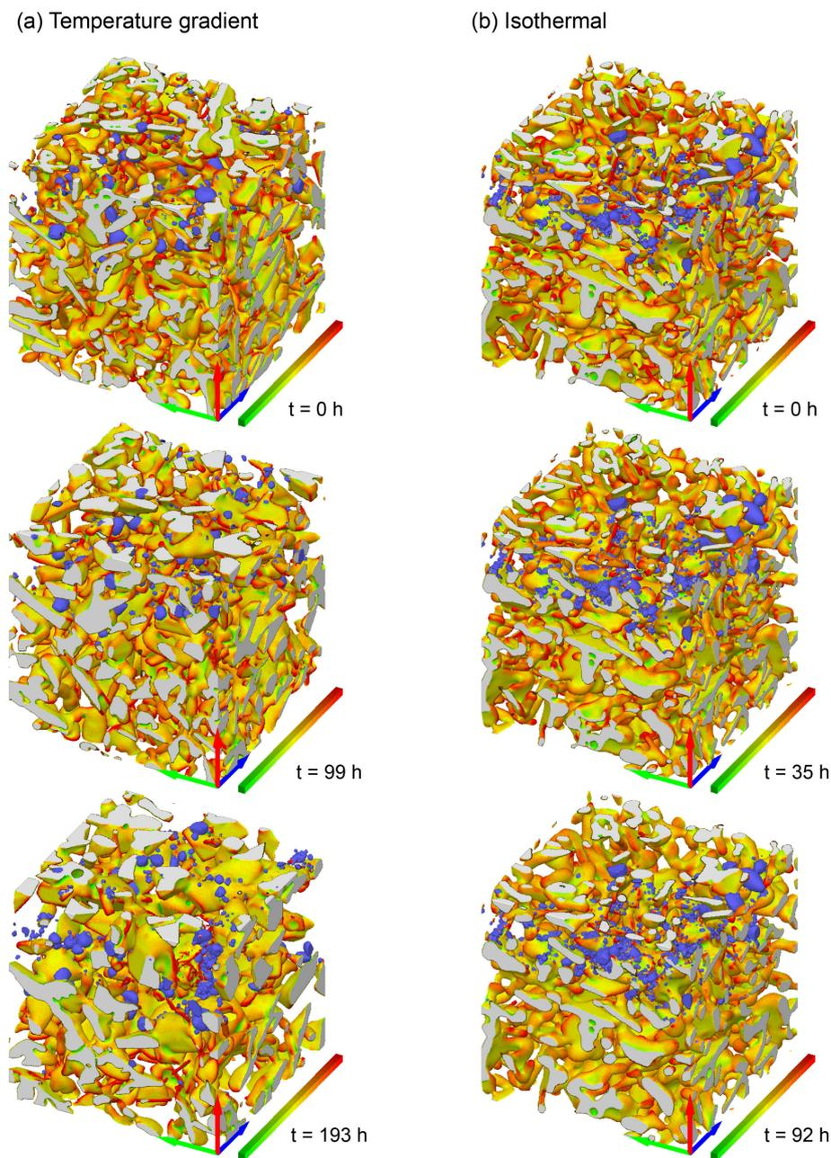
**Figure 1.** Microstructure of the samples at initial, intermediate and final stages. Only subvolumes of size  $3^3 \text{ mm}^3$  are shown with a vertical orientation corresponding to that of the experiment. The color map represents the mean curvature from green ( $-25 \text{ mm}^{-1}$ ) to red ( $+25 \text{ mm}^{-1}$ ) and the colored bar is 3 mm long. The dust particles are shown in blue.
