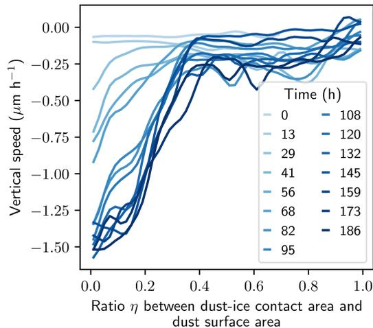
**Figure 5.** Link between dust movement (types 1 and 2) and relative position to ice quantified by  $\eta$  in the temperature gradient experiment.
