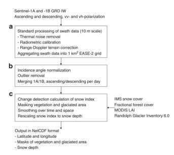
**Fig. 2** Flowchart of the Sentinel-1 processing. **a** The standard backscatter processing techniques are performed using the Google Earth Engine Python's api. **b** Further processing steps, and **c** the application of the retrieval algorithm are performed offline
