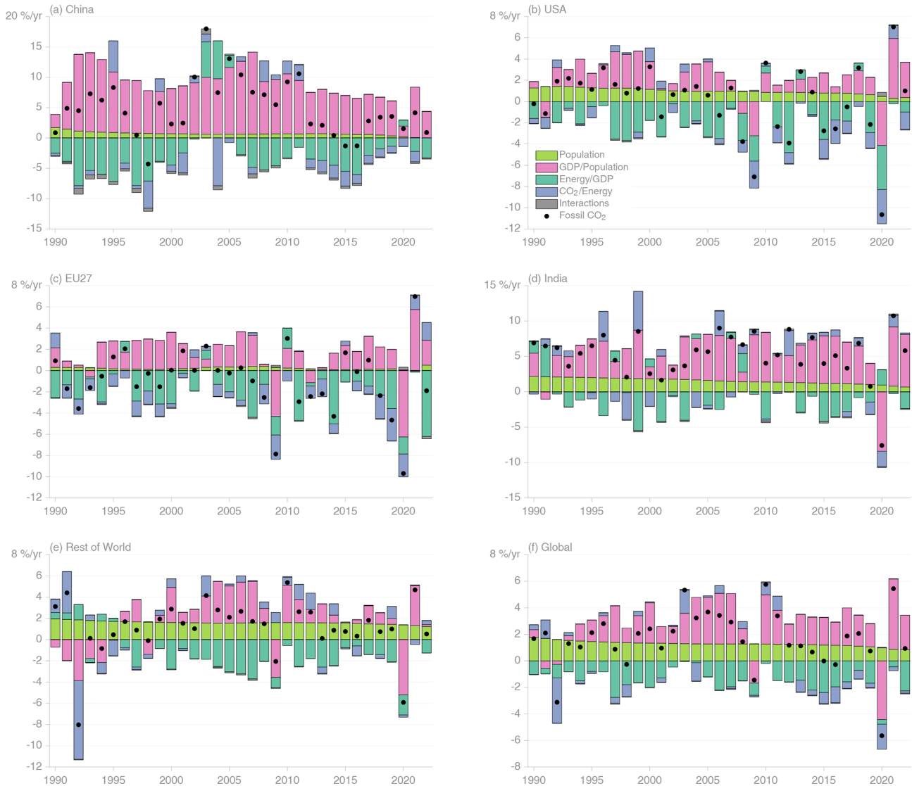
Figure 16. Kaya decomposition of the main drivers of fossil CO 2 emissions, considering population, GDP per person, energy per GDP, and CO 2 emissions per energy unit, for China (a), the USA (b), EU27 (c), India (d), the rest of the world (e), and globally (f). Black dots are the annual fossil CO 2 emissions growth rate; coloured bars are the contributions from the different drivers to this growth rate. A general trend is that population and GDP growth put upward pressure on emissions (positive values), while energy per GDP and, more recently, CO 2 emissions per energy unit put downward pressure on emissions (negative values). Both the COVID-19-induced drop during 2020 and the recovery in 2021 led to a stark contrast to previous years, with different drivers in each region. The EU27 had strong energy per GDP improvement in 2022.
